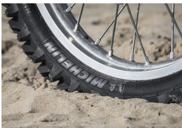
A Tube Type (TT) rim: the spokes pierce the rim in the centre.
